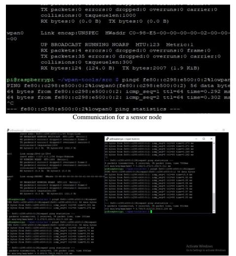
Communication between two sensor nodes using 6LoWPAN protocol
