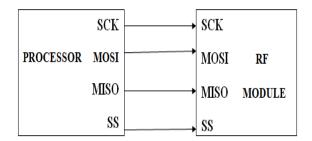
Interfacing between processor and RF module
